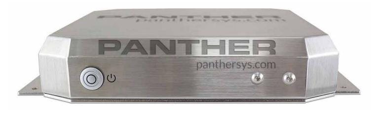
The Waterproof PC design incorporates sealed M12 input/output connectors for power, network, video and peripherals. These sealed ports, a rubber-sealed power button and the absence of a fan and internal power supply inside the thick stainless steel housing make the Waterproof PC a unique solution to the problem of computing in environments where water, corrosive chemicals and dust are prevalent.
